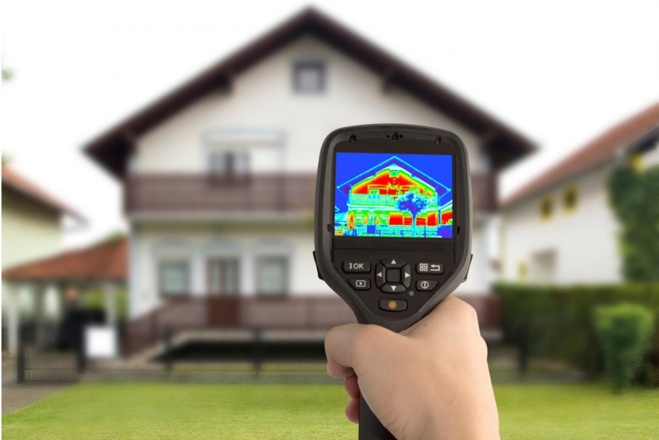
Analyzing household energy efficiency using infrared camera. Photo: Shutterstock.com
