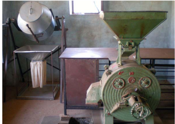
Left: Iron fortification machine. Right: Grain milling machine.
